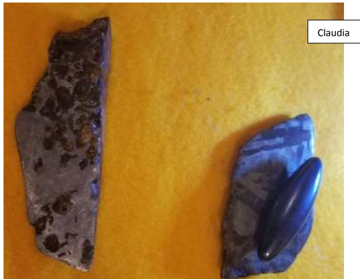
Nickel/Iron meteorite showing "Widmanstätten" pattern on polished surface after etched in acid.
